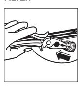
If it takes longer to fill up the washing machine it is time to check the water inlet hose filter it may be clogged. Turn off the water tap. Unscrew the fixing nut of the inlet hose. Remove the filter from the electrovalve and clean it with a hard bristle brush and replace it. Screw on the nut thoroughfully.
